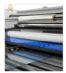
Contact cleaning system of the substrate to laminate with antistatic bar to remove dust from the surface
